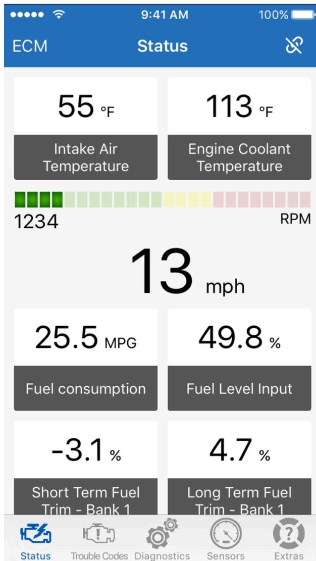
On the top, left corner of the view is the Engine Control Unit (ECU) selection button. Tap the button (in the image labeled ECM) to open the ECU selection. The list contains all OBD2 compliant control units from your car.
